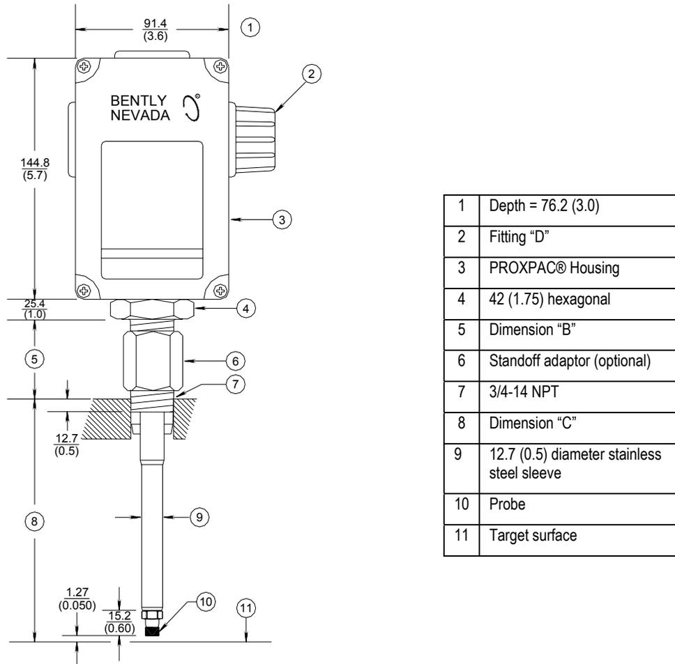
**Figure 2 Dimensions for PROXPAC® Proximity Transducer Assembly**
