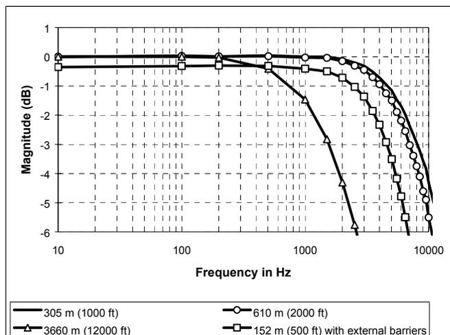
**Figure 1 Typical Frequency Response at 50 mils Gap**
